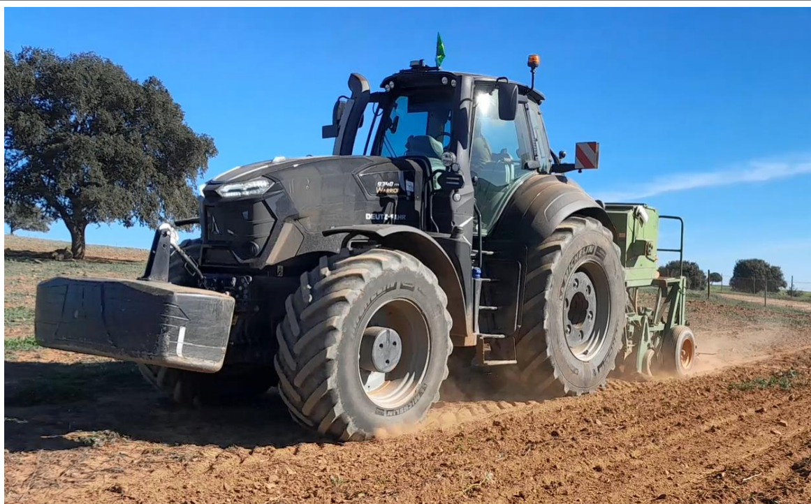
Figure 7: Deutz-Fahr 9340 330 hp tractor set + direct seeder 3,5 m used for direct seeding (Image provided by ADPM).
